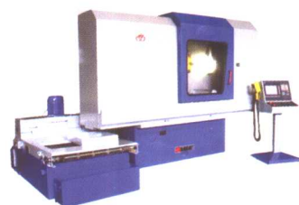
MKL7120X6型数控强力成形磨床
