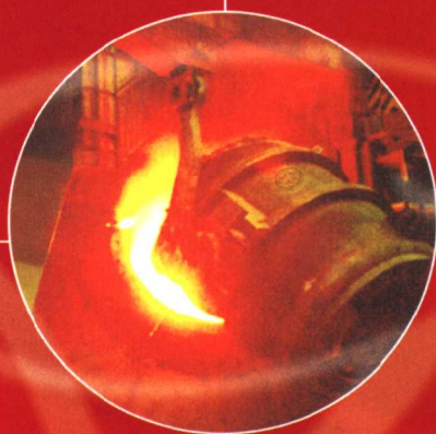
120t 顶底复吹转炉
