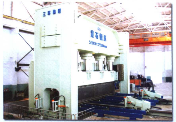
电液伺服数控折弯成型机 (15轴数控) PPF5200/125 (5200t \times 12.5m) PPF3600/120 (3600t \times 12m)
