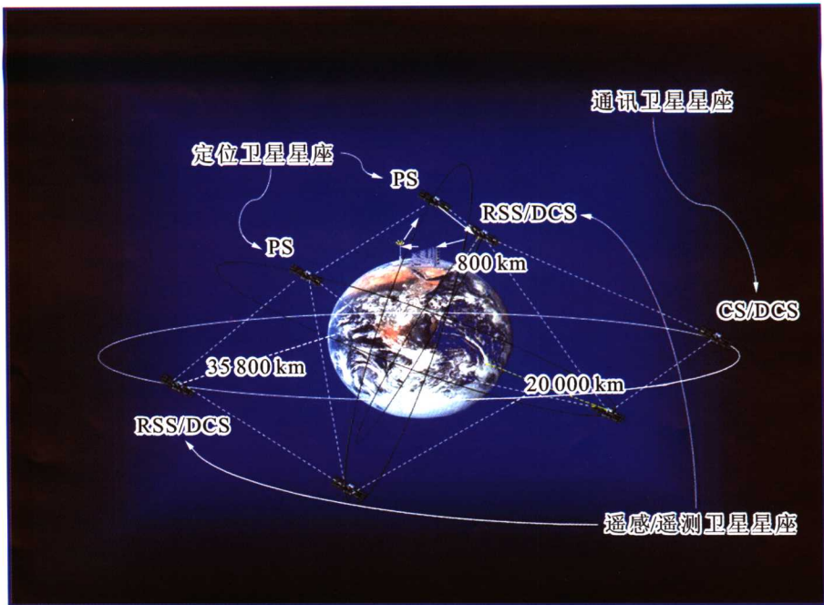
图 1 外层空间人造卫星构成的空间信息网络 Fig.1 The Deep Space Information Network by Satellites
