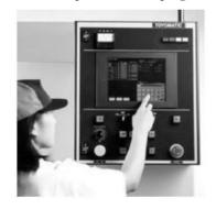
machines to cut and shape precision products, such as automobile, aviation, and machine parts. CNC machines operate by reading the code included in a computer-controlled module, which drives the machine tool and performs the functions of forming and shaping a part formerly done by machine operators<sup>[1]</sup>. CNC machines include machining tools such as lathes, multi-axis spindles, milling machines, laser cutting machines, and wire electrical discharge machines. CNC
