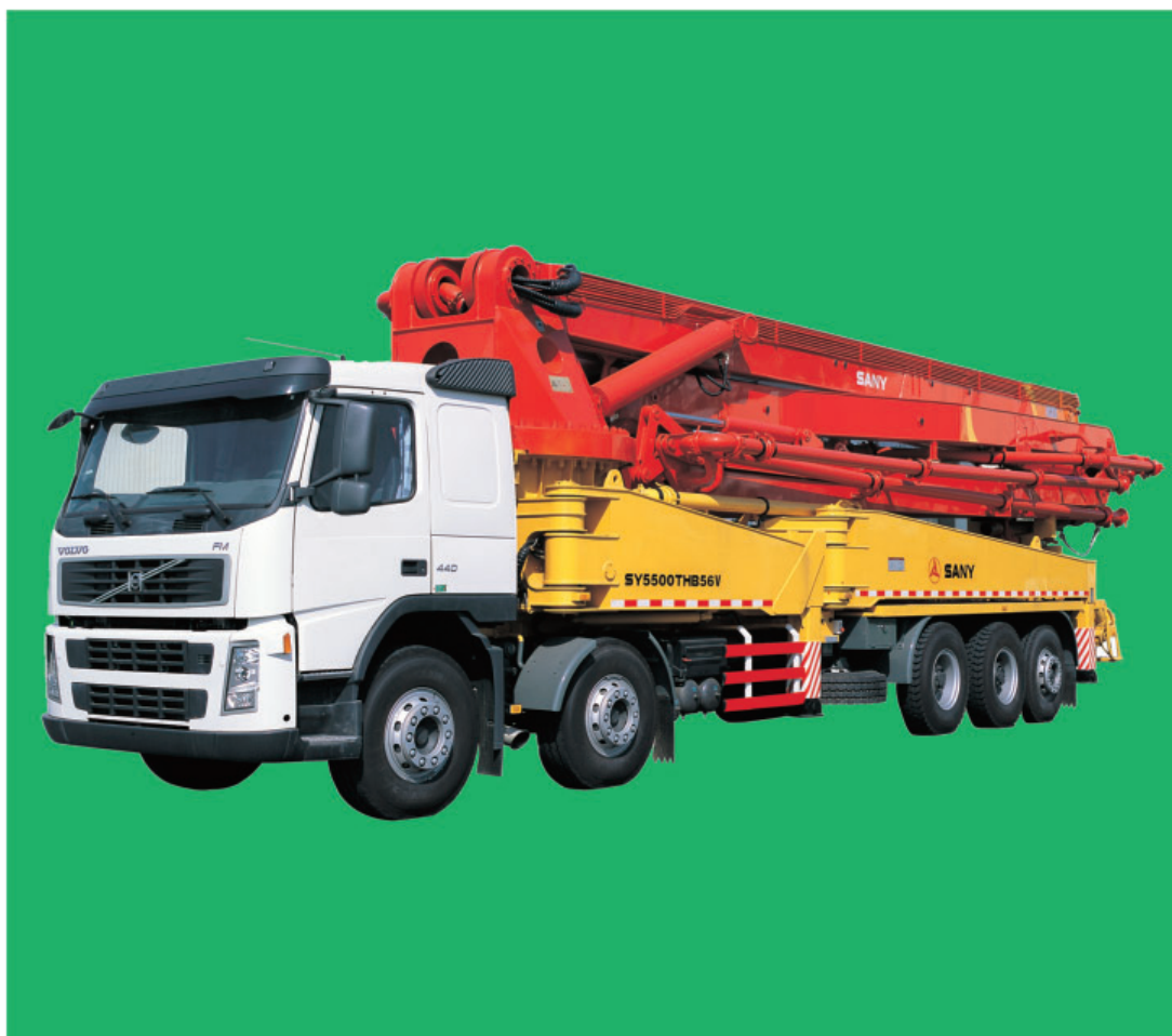
泵车 pump truck
