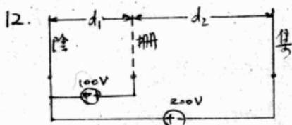
(a)  $F = eE = eV/d = 1.6 \times 10^{-19} \times 100 / 2 \times 10^{-3} = 8 \times 10^{-15} \text{ nC}$  4
