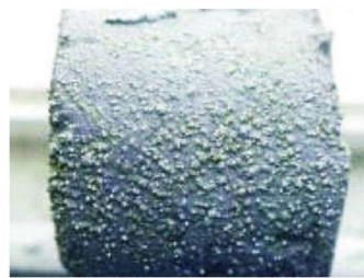
粉末触媒合成棒喷砂后断面 Section of powder catalyst synthesis block after sodablasting
