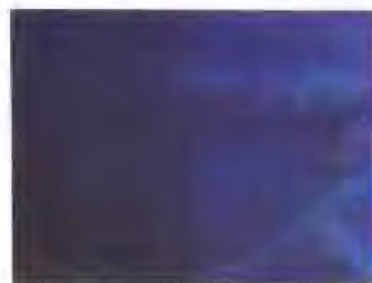
15. 浮色、色分离 Floating and flooding
