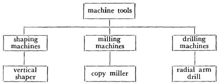
Machine tools can be classified as drilling machines, milling machines and shaping machines. Radial arm drill is an example of drilling machines, and copy miller is an example of milling machines, while vertical shaper is an example of shaping machines.
