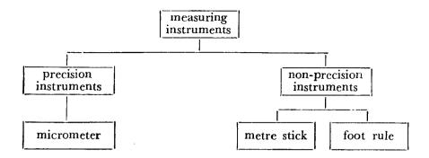
Measuring instruments can be classified as non-precision instruments and precision instruments. Metre stick and foot rule are examples of non-precision instruments. Micrometer is an example of precision instruments.
