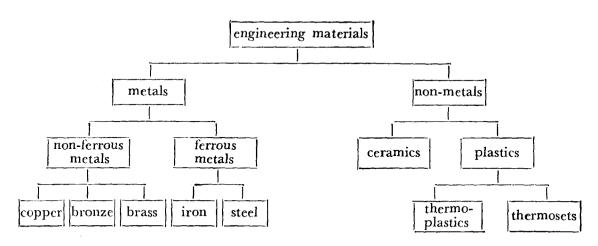
Engineering materials can be classified as non-metals and metals. Non-metals can be classified as plastics and ceramics. Thermosets and thermoplastics are examples of plastics. Metals can be classified as ferrous metals and non-ferrous metals. Iron and steel are examples of ferrous metals, while copper, bronze and brass are examples of non-ferrous metals.
