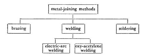
Metals-joining methods can be classified as soldering, welding and brazing. Oxyacetylene welding and electric-arc welding are examples of welding.
