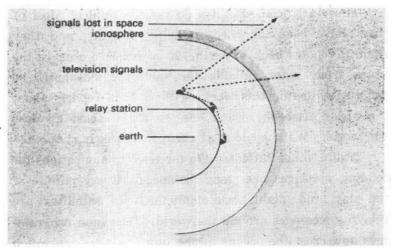
Television waves are not reflected by the ionosphere. They will not go round the curve of the earth unless there are relay stations.
