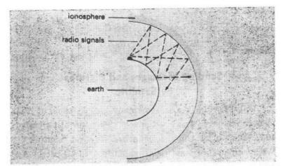
Radio waves are reflected by gases in the ionosphere and can go round the curve of the earth.
