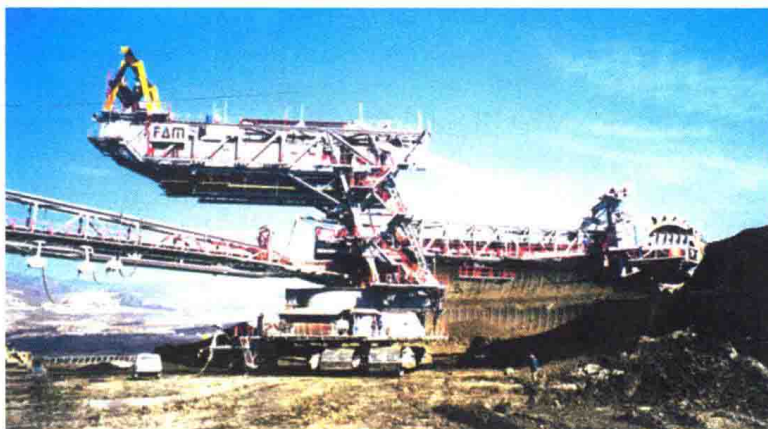
A bucket-wheel excavator is the largest equipment in the world.
