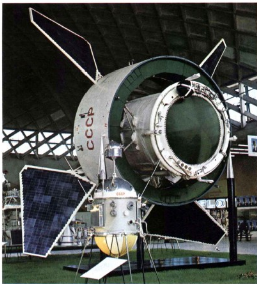
▲ Two Soviet satellites on display at an aerospace exhibition. A craft of the Proton 1 type dwarfs a Cosmos satellite. Proton 1 weighed over 10 tonnes, was unmanned, and made measurements of cosmic rays. The four 'paddles' are solar panels, which turn the energy of sunlight into electrical energy. Many satellites were launched in the Cosmos series. They studied the electrical and magnetic fields of the Earth, cosmic rays and radiation from the Sun
