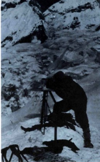
Surveying on a plane table to map the area, during an expedition to the Himalayan mountains in 1957. The table can be adjusted to level it on such uneven ground, so that it is exactly horizontal.
