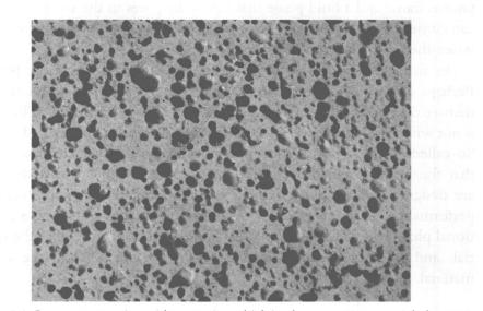
**Figure 1.1** Porous composite oxide ceramics, which is a low-porosity material, shown as a cross-sectional image.
