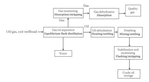
Following the order of events using this flow sheet, one can determine the function of every piece of equipment involved in an oil field process design, highlighted in bold. The immediate next step is the determination of the size and the type of equipment needed to carry out the physical changes, using the unit operations principle underlying this process. Remember that the fundamentals pertaining to a given unit operation are the same regardless of its application, hence unit operation.
