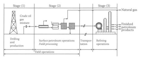
Petroleum and gas field processing operations, referred to as surface petroleum operations (SPO), cover the myriad procedures required to handle the crude oil mixture between the well head and the delivery points for refining operations and other usages. xx Introduction
