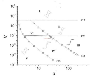
Figure 1.3 Zone diagram of cyclic voltammetric behavior at microelectrode arrays. *d* is the center-to-center distance of individual electrodes in the array (measured in units of *r*), *V* is the dimensionless scan rate (see Eq. 1.3). Note, this is for a hexagonal arrangement. (Reproduced from Ref. [12], copyright 2005, American Chemical Society.)
