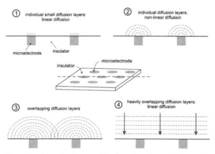
Figure 1.1 Schematic diagram of the four categories a diffusion profile may belong to an array of microelectrodes (reproduced from Ref. [11] with permission from Elsevier).
