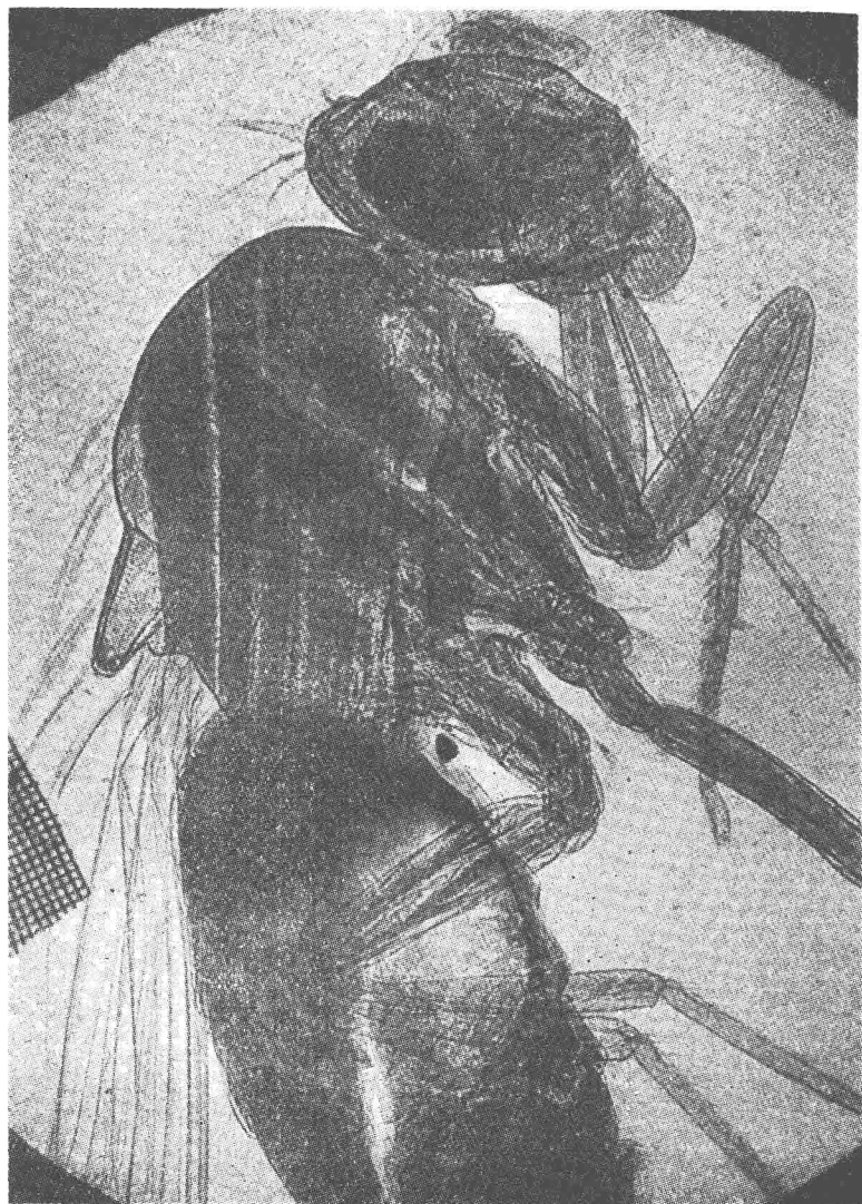
Courtesy Coslett and Nison Micro-radiograph of Drosophila melanogaster (fruit fly), freeze-dried. Primary magnification \times 20 ; enlargement factor \times 7.5 ; total magnification \times 150 . The pattern in the upper left corner is a portion of a silver grid, 1500 meshes per inch.
