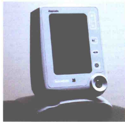
Fig. 1-3 Fifth-generation (frequency-type) apex locator.
