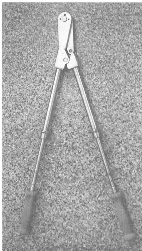
Fig. 1.7. Specialist large diameter wire cutters using shearing rather than a cutting action.
