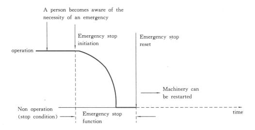
Figure 1 Graphical representation of emergency stop function
