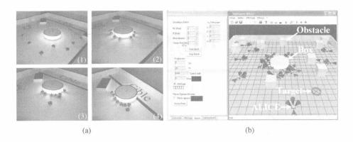
FIGURE 1 (See color insert) (a) Experimentation of the proposed control architecture with 8 mini-robots ALICE pushing a cylindrical object to a final assigned area; (b) MiRoCo simulator.
