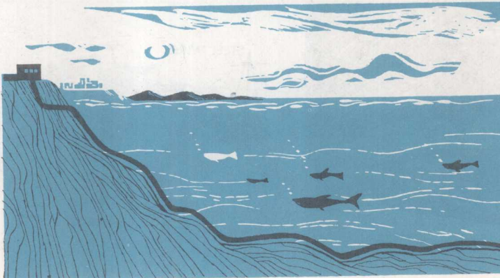
Left: Cables that carry telegraph and telephone messages are laid under the oceans between continents. Right: Cross-sectional view of a submarine telephone cable. The center copper wire is only one-tenth of an inch in diameter and can carry 36 voices at the same time. The many outer layers are for protection.
