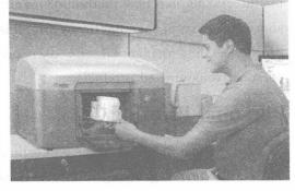
Systems. The original aim was to rapidly create prototypes for manufacturers using large machines, but the technology has been greatly improved over the years. It has also gotten cheaper to the point that there are now personal 3D printers available in the mainstream market.
