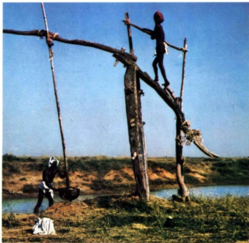
▲ A simple apparatus for raising water in monsoon areas such as India.
