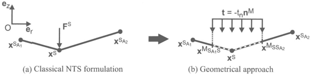
Fig. 2: Node to surface with geometrical area regularization formulation. (a) Classical NTS formulation and (b) geometrical approach.
