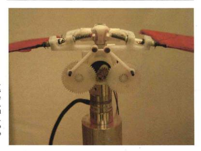
together. The rotation about the wing axis is accomplished by a cam-and-follower mechanism. Cam mechanisms are discussed in Chapter 10.
