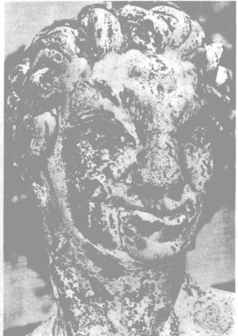
Fig. 7. Head of a bronze statue in Munich showing the effects of air pollution
