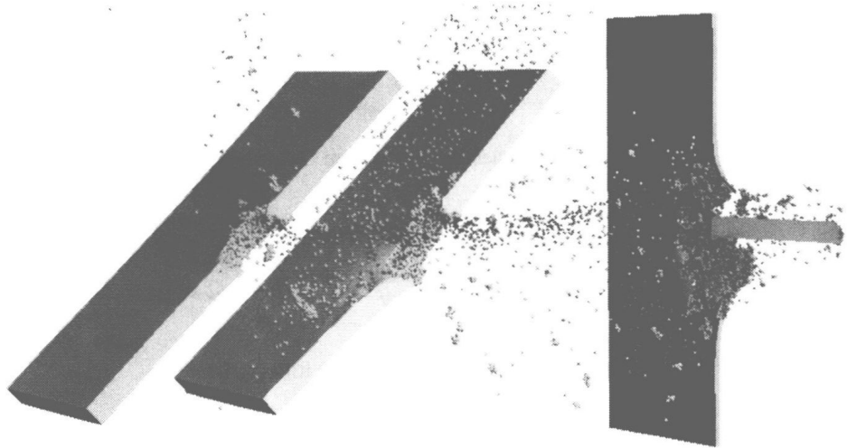
Figure 3: Projectile perforation through spaced plate array.
