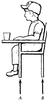
FIG. 1.1 The floor exerts forces on the chair.
