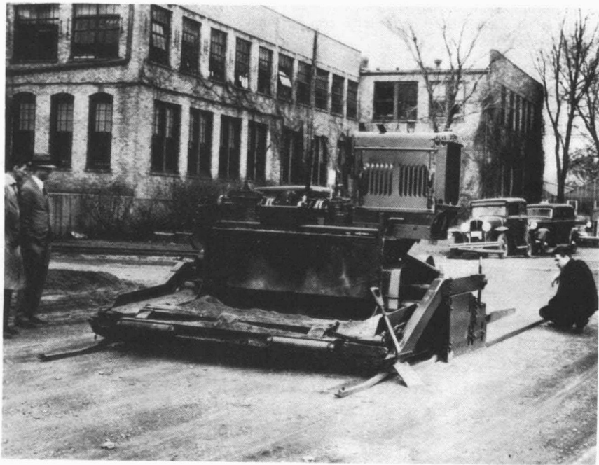
FIG. 1—1933 model self-propelled paver with floating screed.
