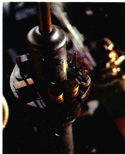
Although Londoners refer to the familiar clockface (top) as Big Ben, the name properly belongs only to the great bronze hour-bell. The clock’s 13-foot pendulum is adjusted to keep perfect time by adding and removing coins from two piles of pennies (bottom) that are balanced on the pendulum weight.
