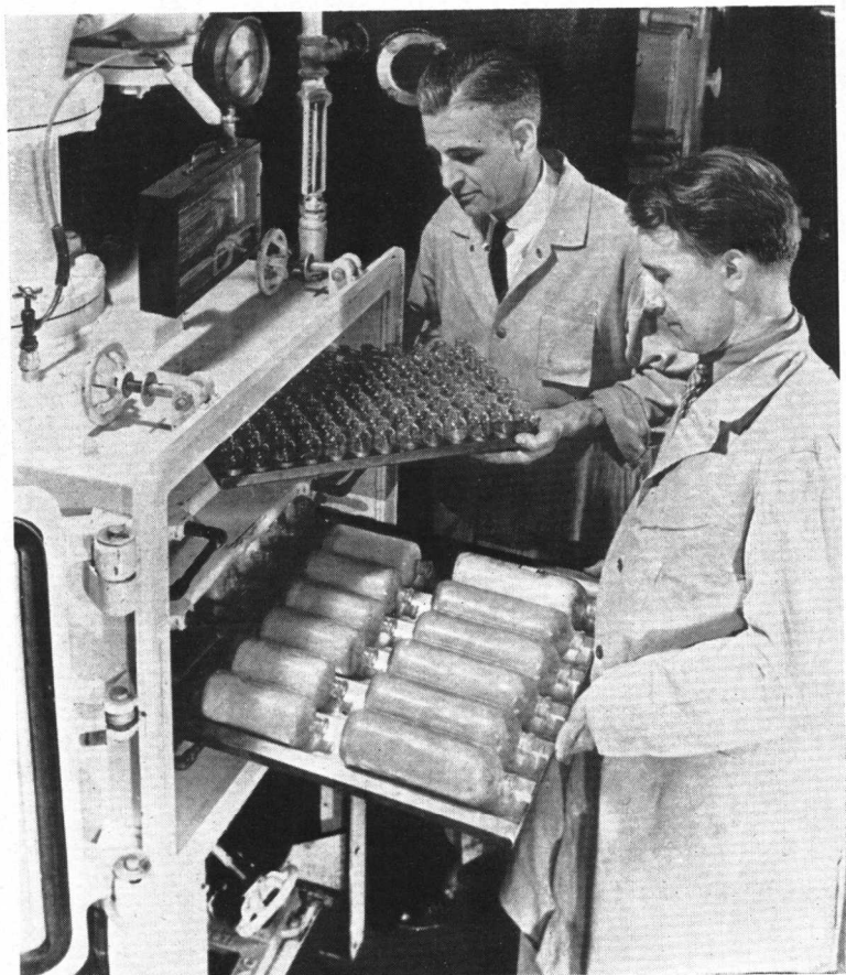
FIG. 2. Drying Chamber being loaded with racks for supporting plasma bottles and for supporting small vials of antibiotics. No protective covering is provided in this case.
