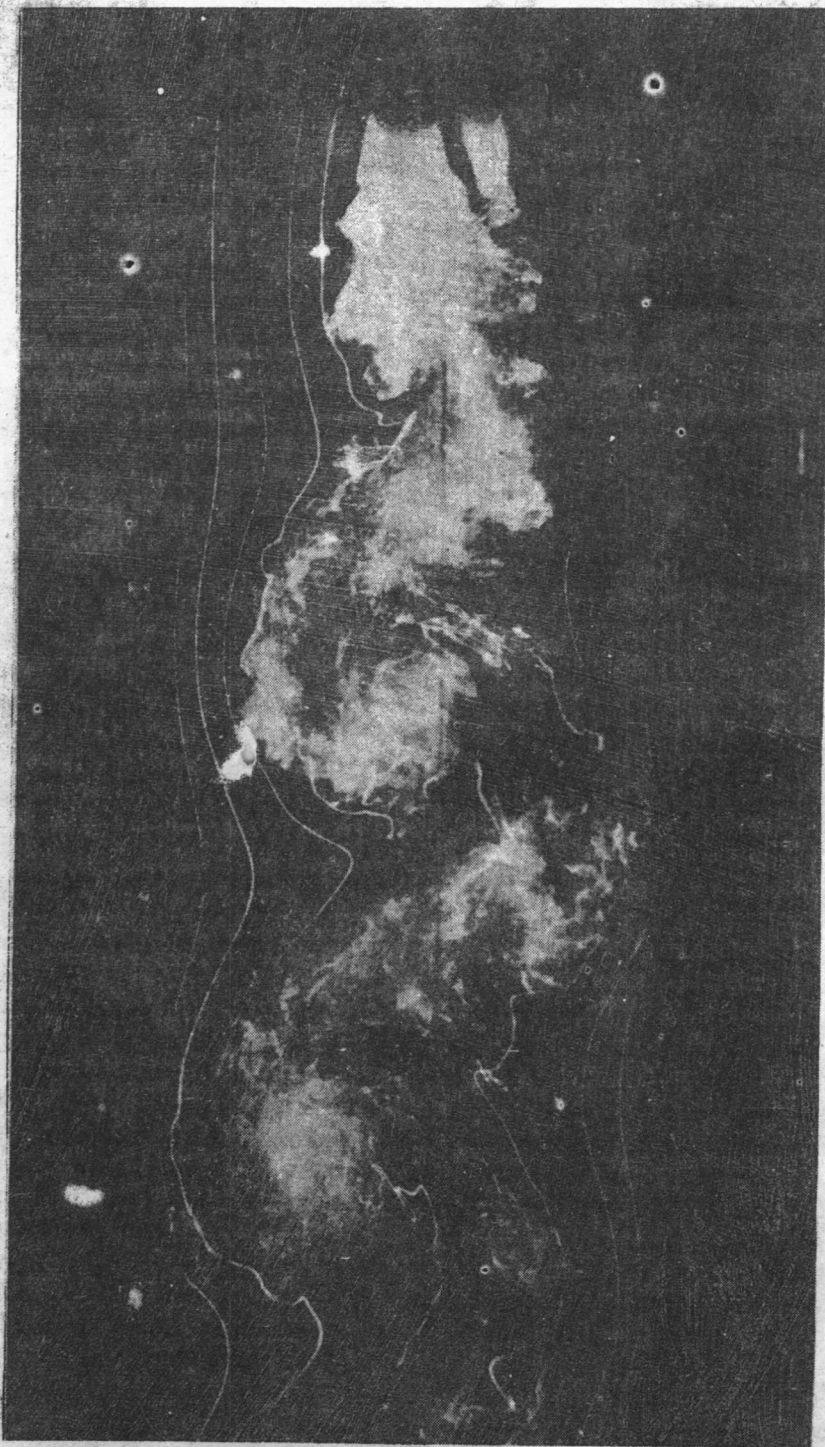
Figure 1-1 Turbulent wake in the flow past a circular cylinder [courtesy of R. Dumas].
