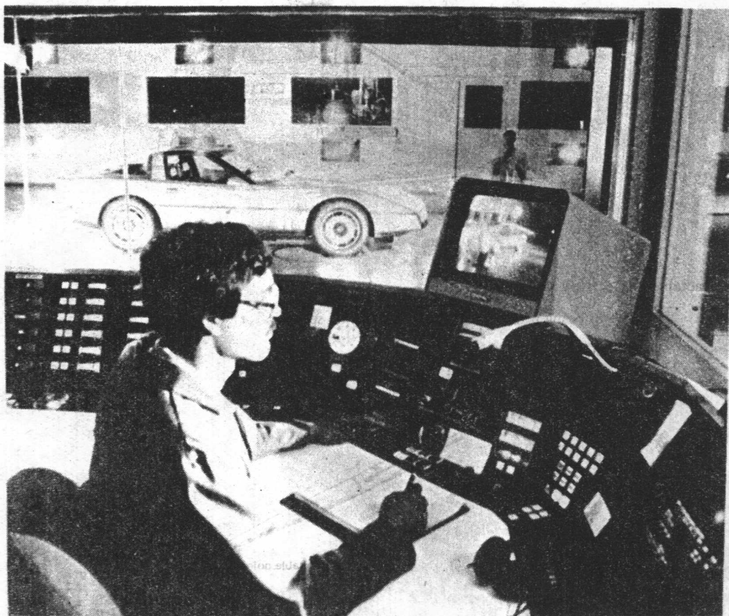
An engineer checks drag coefficient numbers in the test section control room of the wind tunnel.
