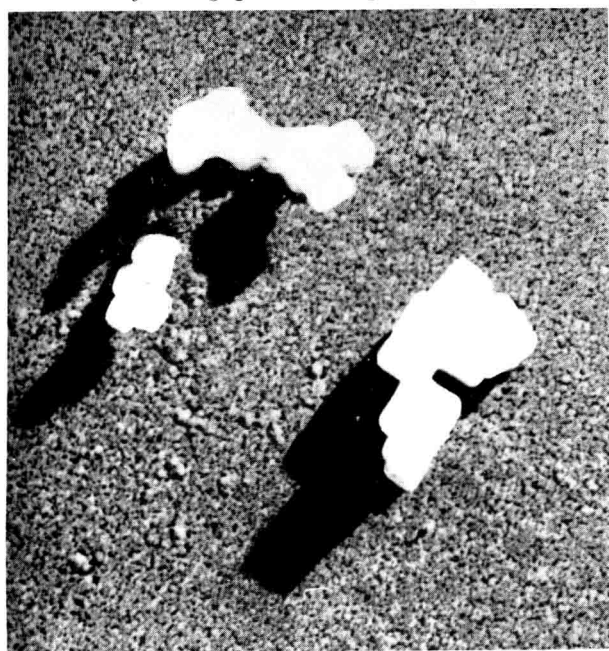
Fig. 4.—Magnesium oxide crystals, shadowcast with gold at \cot^{-1}2 . ( \times 31,000 )
