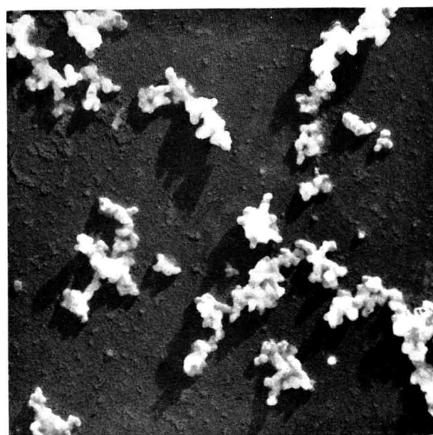
Fig. 5.—Carbon black particles, shadowcast with palladium gold alloy at \cot^{-1}2 . ( \times 30,000 )
