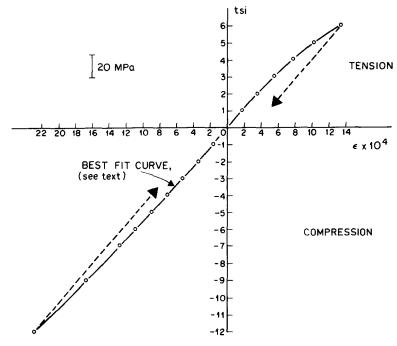
Fig. 2. Only by testing very long bars could Hodgkinson obtain measurable strains in compression.
