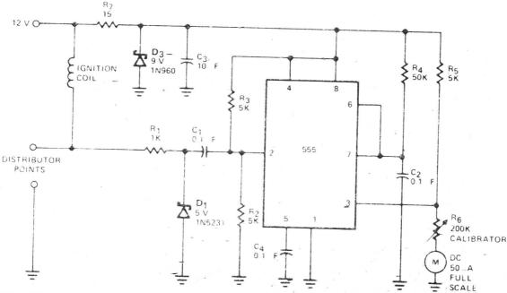
DISTRIBUTOR-POINT TACHOMETER—555 timer receives its input pulses from distributor points of car. When timer output (pin 3) is high, meter receives calibrated current through R<sub>6</sub>.
