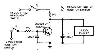
HEADLIGHTS-ON ALARM—Designed for cars in which headlight switch is nongrounding type, providing 12 V when closed. When both light and ignition switches are closed, transistor is saturated and there is no voltage drop across it to drive buzzer. If ignition switch is open while
