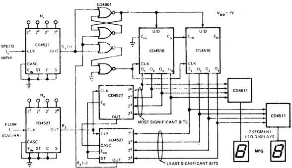
MILEAGE COMPUTER—Fuel consumption in miles per gallon is continuously updated on 2-digit LED display. Entire system using CMOS IGs can be built for less than \$25 including gas-flow sensor and speed sensor, sources for which are given in article along with operational details.
