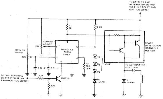
VOLTAGE REGULATOR—Timer and power Darlington form simple automobile voltage regulator. When battery voltage drops below 14.4
