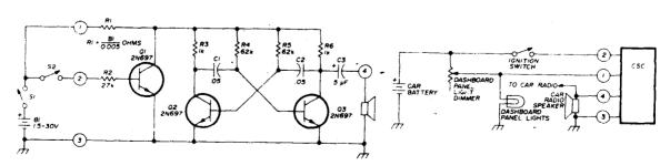
HEADLIGHT REMINDER—Uses basic oscillator consisting of Q2 and Q3 arranged as collector-coupled astable MVBR. Power is taken from collector of Q1 which acts as switch for Q2 and Q3. With S1 closed and S2 open, oscillator operates. Closing S2 saturates Q1 and stops oscillator. When used as headlight reminder for negative-
