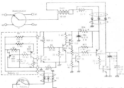
COLD-WEATHER IGNITION—Multispark electronic ignition improves cold-weather starting ability of engines in arctic environment by providing more than one spark per combustion cycle. Circuit uses UJT triangle-wave generator Q1, emitter-follower isolator Q2, wave-shaping Schmitt trigger Q3-Q4, three stages of square-wave amplification Q5-Q7, and output switch-
