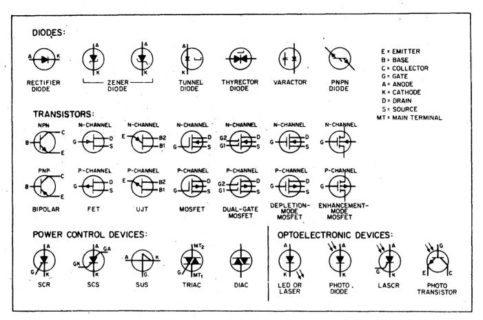
The commonest forms of the basic semiconductor symbols are shown here. Leads are identified where appropriate, for convenient reference. Minor variations in symbols, particularly those from foreign sources, can be recognized by comparing with these symbols while noting positions and directions of solid arrows with respect to other symbol elements.
