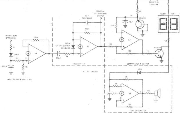
HIGH-SPEED WARNING—Audible alarm tone generator drives warning loudspeaker to supplement 2-digit speed display that can be set to trip when vehicle speed exceeds 55-mph legal limit. Engine speed signal is taken from primary of sperk coll. Switch in transmission activates circuit only when car is in high gear. All func-
