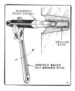
Figure 14. Removing broken stud with cold chisel.
