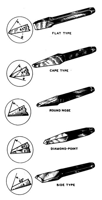
Figure 9. Types of cold chisel, and average cutting-edge angle of each.
