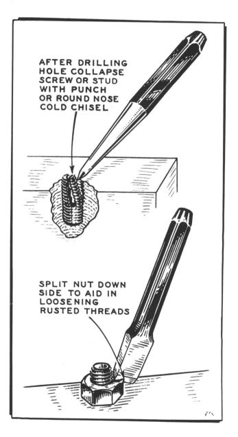
Figure 15. Removing broken or rusted screws and nuts with cold chisel.
