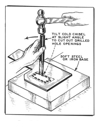
Figure 11. Cutting slots or holes in metal.
