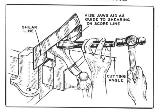
Figure 10. Cutting metal with a cold chisel.
