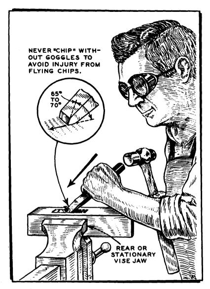
Figure 12. Always drive flat chisel toward the stationary jaw vise.
