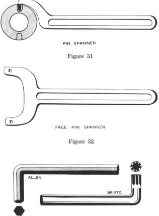
Special Wrenches. Figure 33 shows the Allen-type wrench. Its six-sided shaft fits into the hollow hexshaped recess of setscrews and capscrews. This wrench comes in sizes from 1/8 to 3/4 in., and the
