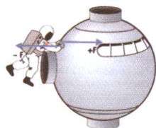
Figure 4.8 The astronaut pushes on the spacecraft with a force +F . According to Newton's third law, the spacecraft simultaneously pushes back on the astronaut with force -F .
