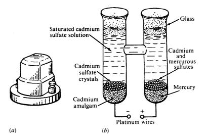
Fig. 1.1 Appearance (a) and construction (b) of a Weston standard cell.
