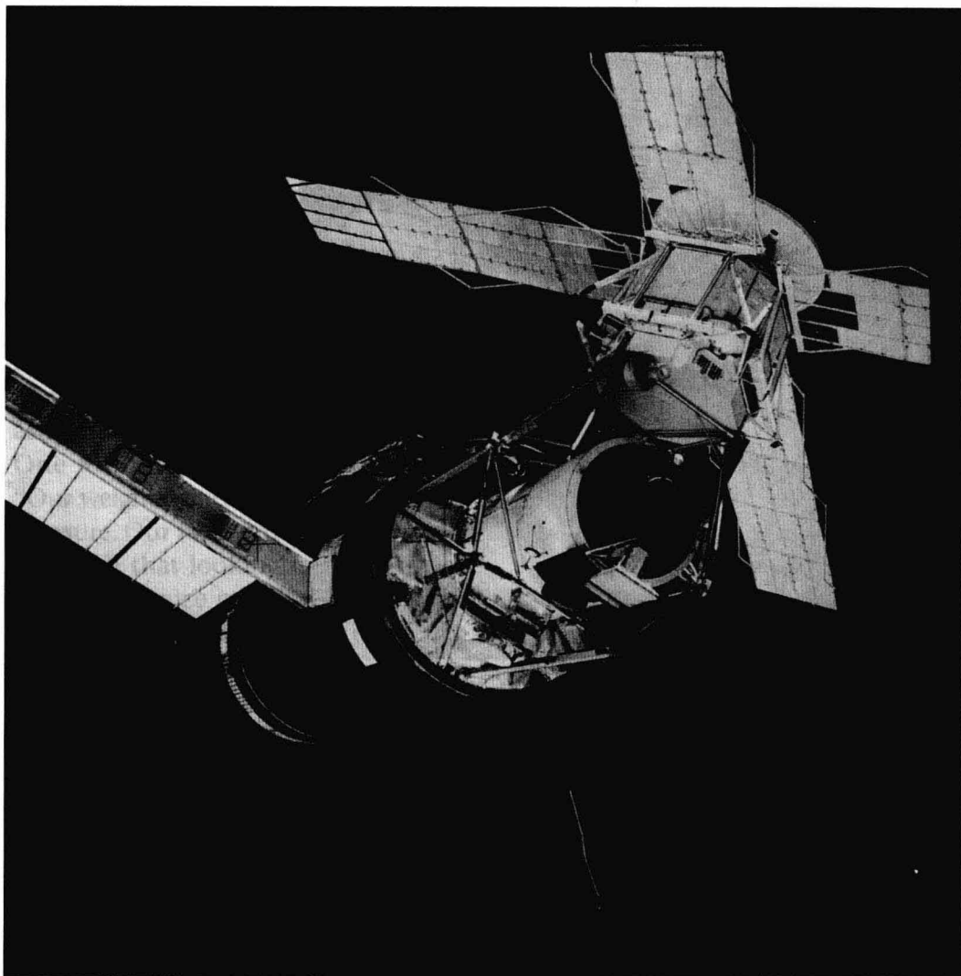
Skylab space station, as seen from the command module. The protrusions are huge solar panels attached to the space station.
