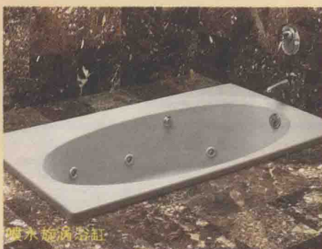
ROMA 5 1/2 WHIRLPOOL. 1524mmx1067mmx406mm. Acrylic. Six multi-directional jets. Oval bathing well with slip-resistant surface, back support, and beveled headrest.
