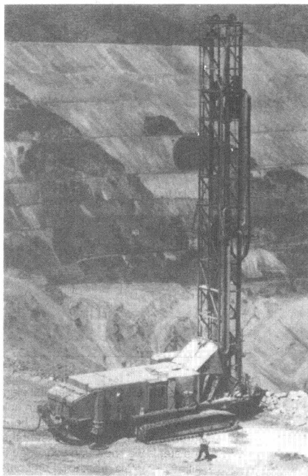
FIGURE 1.1a Open-pit mining showing a 12 1/4-in. rotary drill in the foreground. (Kennecott Copper Corporation photograph by Don Green)
