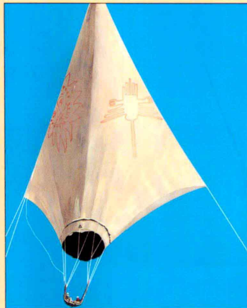
A two-man crew tested Condor I, sitting on a cradle made from bundles of reeds.
