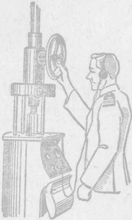
Operating position of a marine radio direction finder.
