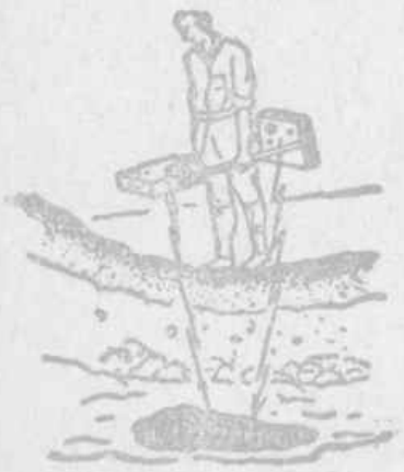
Metal detector used for locating mineral lode.
