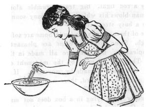
The prongs move only a little way, and they move very fast. It is hard to see that they are vibrating. The picture above shows a good way of finding out that the prongs are vibrating. Notice the drops of water that the fork is flipping out as it moves back and forth. If you try this experiment for yourself, be careful to hold the fork so that just the ends touch the water.
