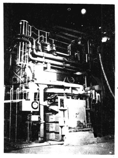
Large electric arc furnace used in steel production. Such loads on the electricity supply system often require reactive power control equipment of the type described in Chapter 9.
