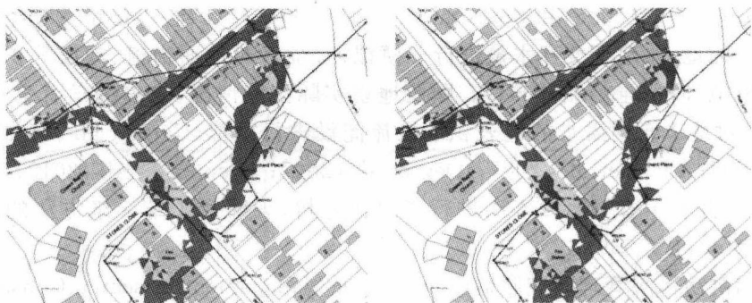
图 1.5 InfoWorks CS 2D 耦合排水设施的淹没模拟(Alitt et al., 2009)
