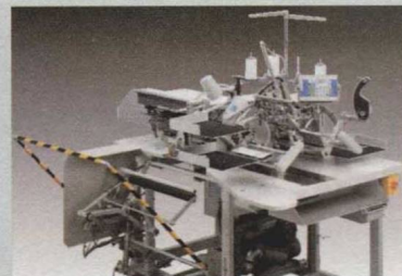
745-35-10 B 开直袋或 (选购) 开斜袋, 袋盖袋和手巾袋 Runstitching of straight or optionally slanted piped pockets, flap pockets and welt pockets
