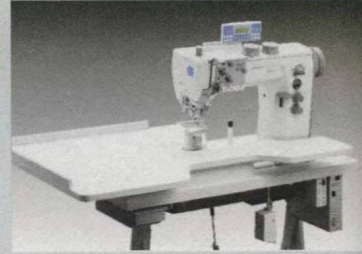
680 缝合大身衬里和同步修剪袖窿 Attaching body lining and simultaneous trimming of armholes
